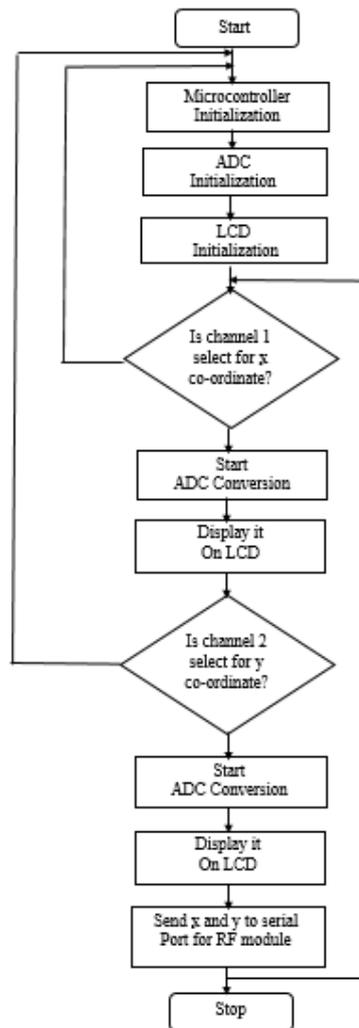
Fig. 2. Flowchart of working flow of pen module
