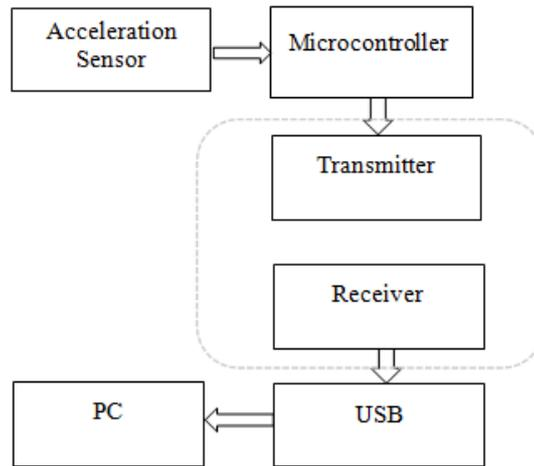
Fig 1: Block Diagram of Electro Pen system
