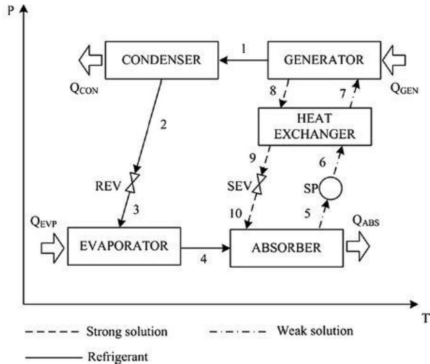
Fig. 1. Schematic diagram of a single-effect LiBr-H<sub>2</sub>O ARS.
