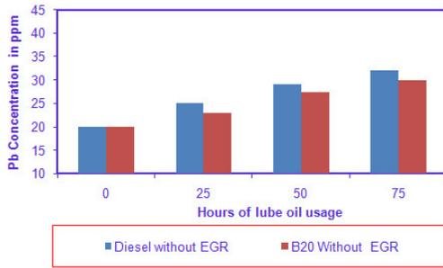
**Fig 7. Lead Concentration Vs Hours of lube oil**
