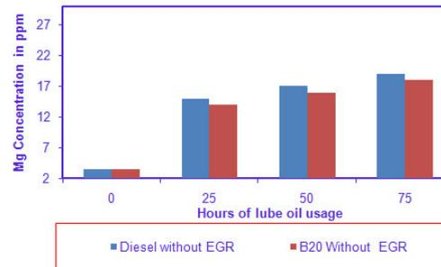
**Fig 6. Magnesium Concentration Vs Hours of lube oil**
