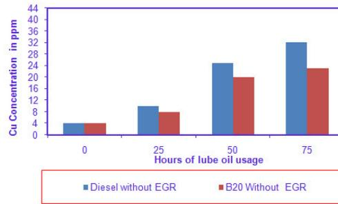
**Fig 4. Copper Concentration Vs Hours of lube oil**
