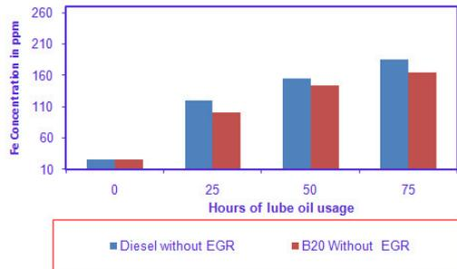
**Fig 5. Iron Concentration Vs Hours of lube oil**
