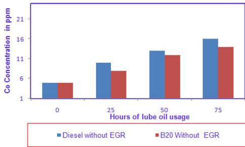
**Fig 3. Cobalt Concentration Vs Hours of lube oil**
