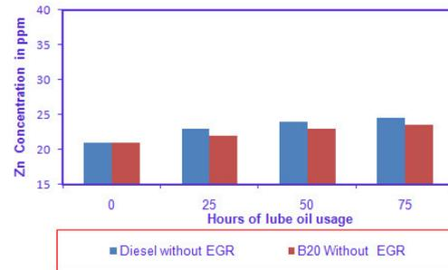
**Fig 8. Zinc Concentration Vs Hours of lube oil**
