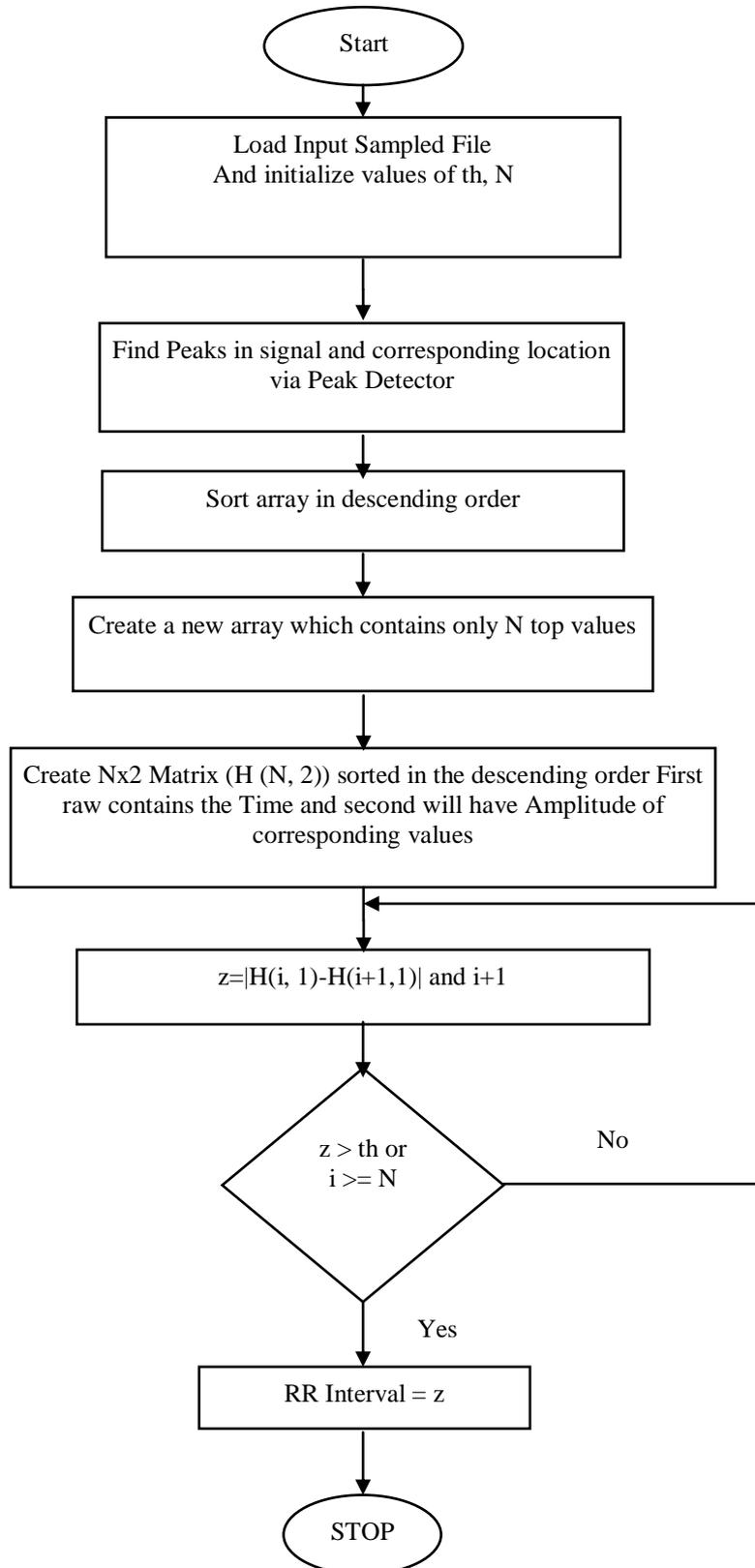
Figure 3: Flow Chart of Automatic RR interval Measurement
