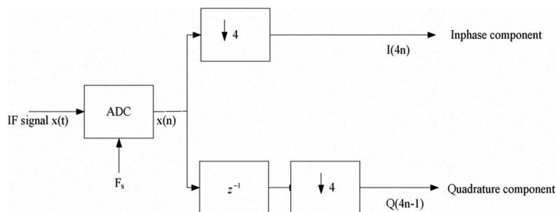
**Figure2. Block diagram of digital down converter**
