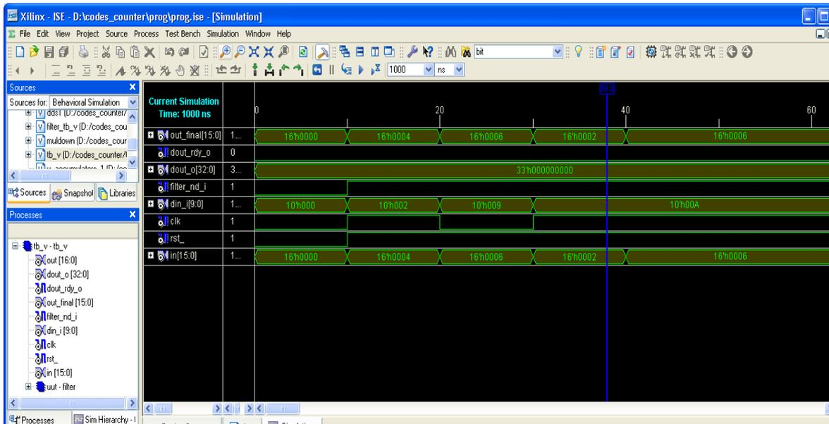
Figure4. Simulation of Digital up/down converter on WCDMA signal
