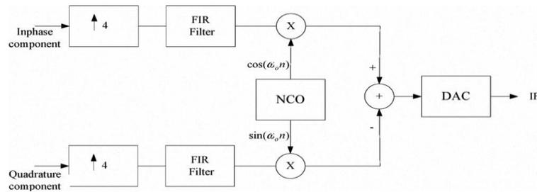
**Figure1. Block diagram of digital up converter**
