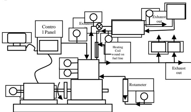
Airflow measurement was done by the conventional method u-tube manometer as well as by air intake DP unit present in the control panel. Engine speed was sensed and indicated by an inductive pickup sensor in conjunction with a digital RPM indicator, which was a part of eddy current dynamometer controlling unit. A strain gauge type load cell mounted beneath the dynamometer arm measures the load and signals are interfaced with ADC card to give load in kg. Temperature sensors of RADIX Pvt. Ltd. make
