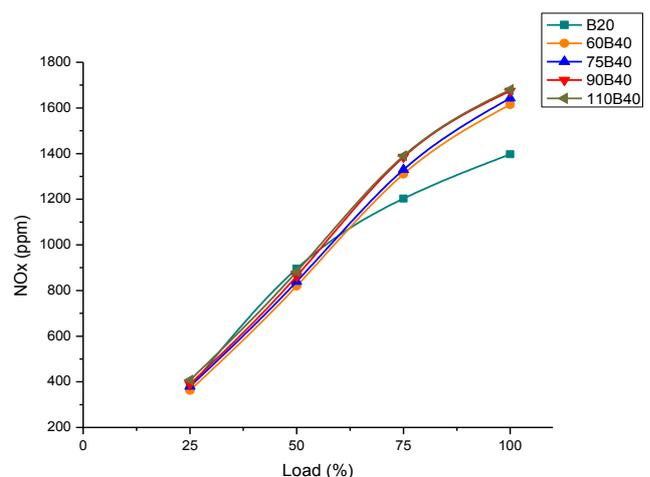
Figure 4. Variation of NOx for B40 blend for different preheating temperature and B20
