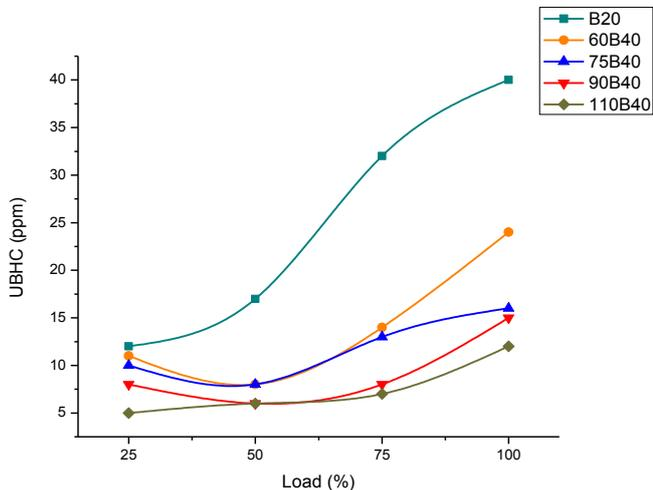
Figure 3. Variation of UBHC of B40 blend for different preheating temperature and B20
