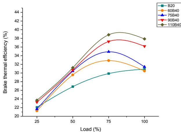
Figure 1. Variation of BTE for B40 blend at different preheating temperature and B20
