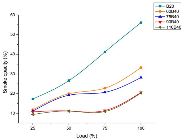
Figure 5. Variation of smoke opacity for B40 blend for different preheating temperature and B20
