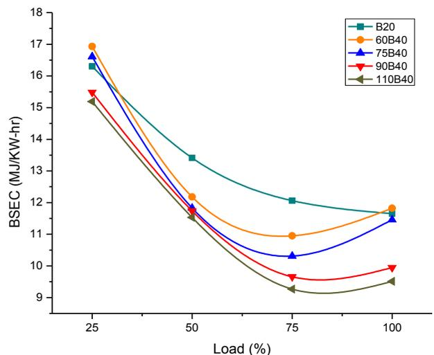
Figure 2. Variation of BSEC for B40 blend at different preheating temperature and B20
