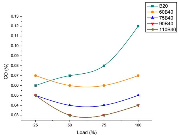
Figure 6. Variation of CO for B40 blend for different preheating temperature and B20
