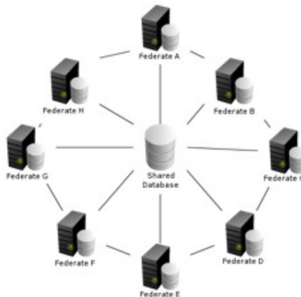
**Fig. 1(b): Hybrid P2P Architecture**
