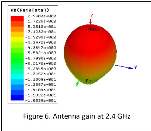
Figure 6. Antenna gain at 2.4 GHz
