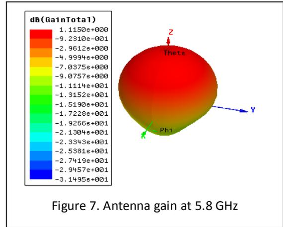
Figure 7. Antenna gain at 5.8 GHz
