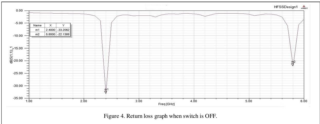
Figure 4. Return loss graph when switch is OFF.
