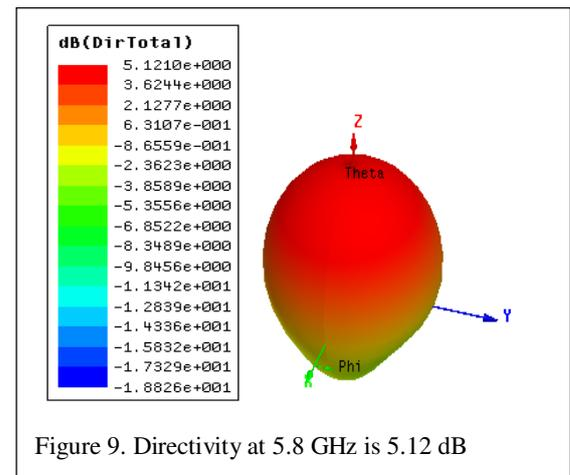
Figure 9. Directivity at 5.8 GHz is 5.12 dB
