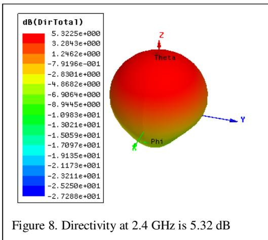
Figure 8. Directivity at 2.4 GHz is 5.32 dB
