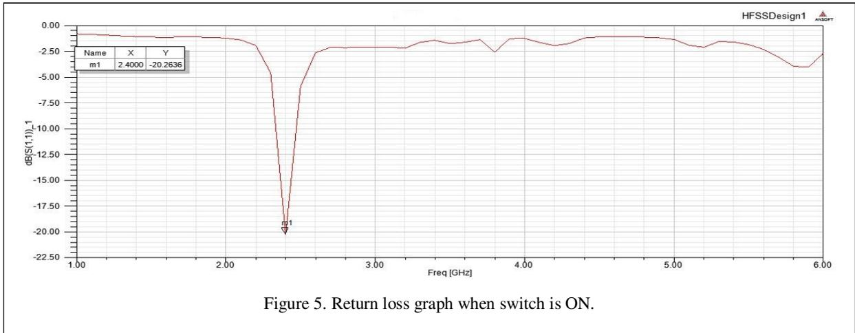
Figure 5. Return loss graph when switch is ON.
