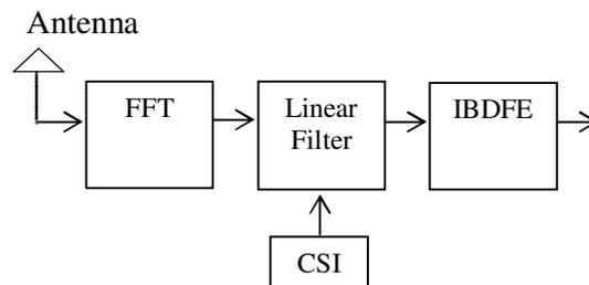
Fig. 2 IBDFE Based Receiver structure.
