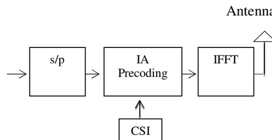
Fig. 1 IA Precoding Based Transmitter.
