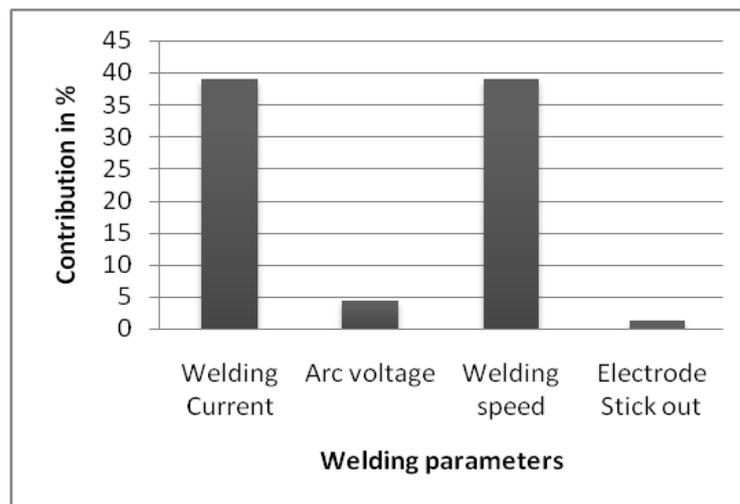
Figure.1.2 Influence of process parameters on bead penetration.
