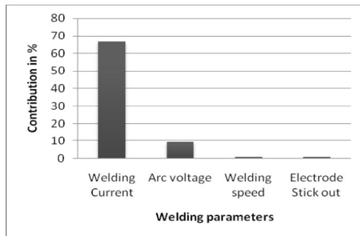
Figure. 1.1 Influence of process parameters on bead width.
