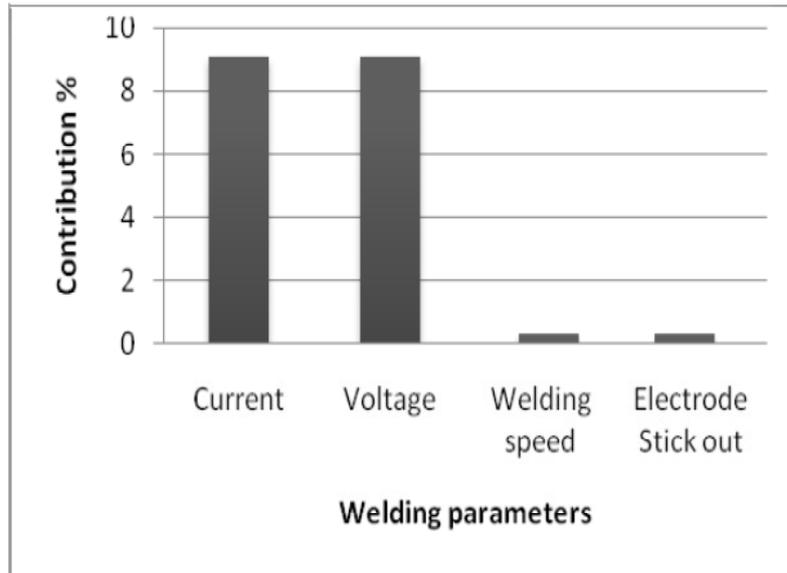
Figure.1.3 Influence of process parameters on weld reinforcement.
