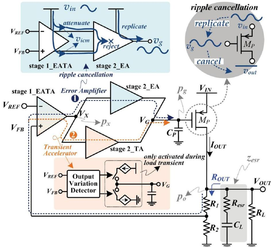
Figure 2. Block Diagram of Proposed LDO regulator
