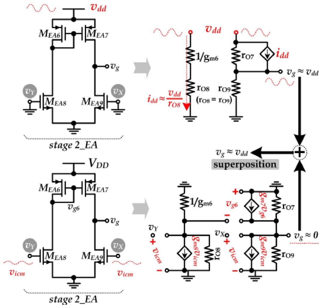
Figure 4. Low-frequency, small-signal model of the EA output stage (stage 2\_EA) for ripple cancellation analysis
