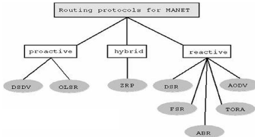
Figure 3. Types of routing protocol
