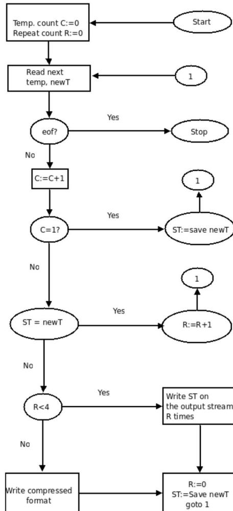
Figure 3. Data compression algorithm flow chart
