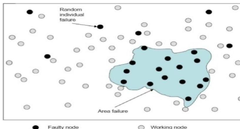
**Figure 4. Fault node**
