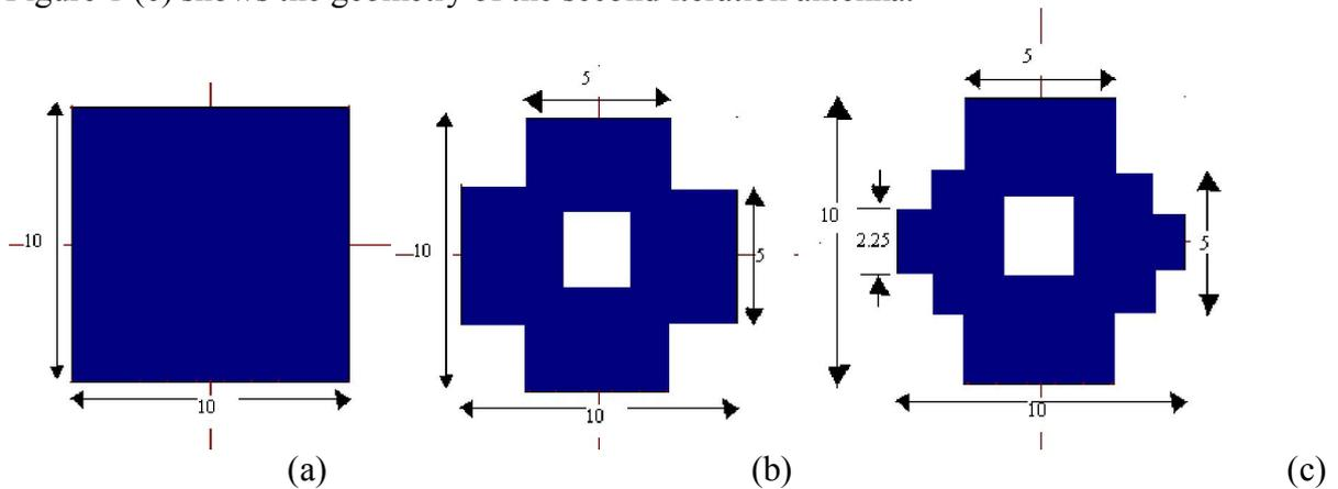
Figure 1 (a) Square patch antenna (b) First iteration (c) Second iteration
