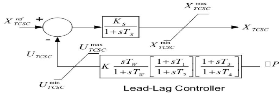
Fig. 4 Structure of a simple TCSC POD controller.
