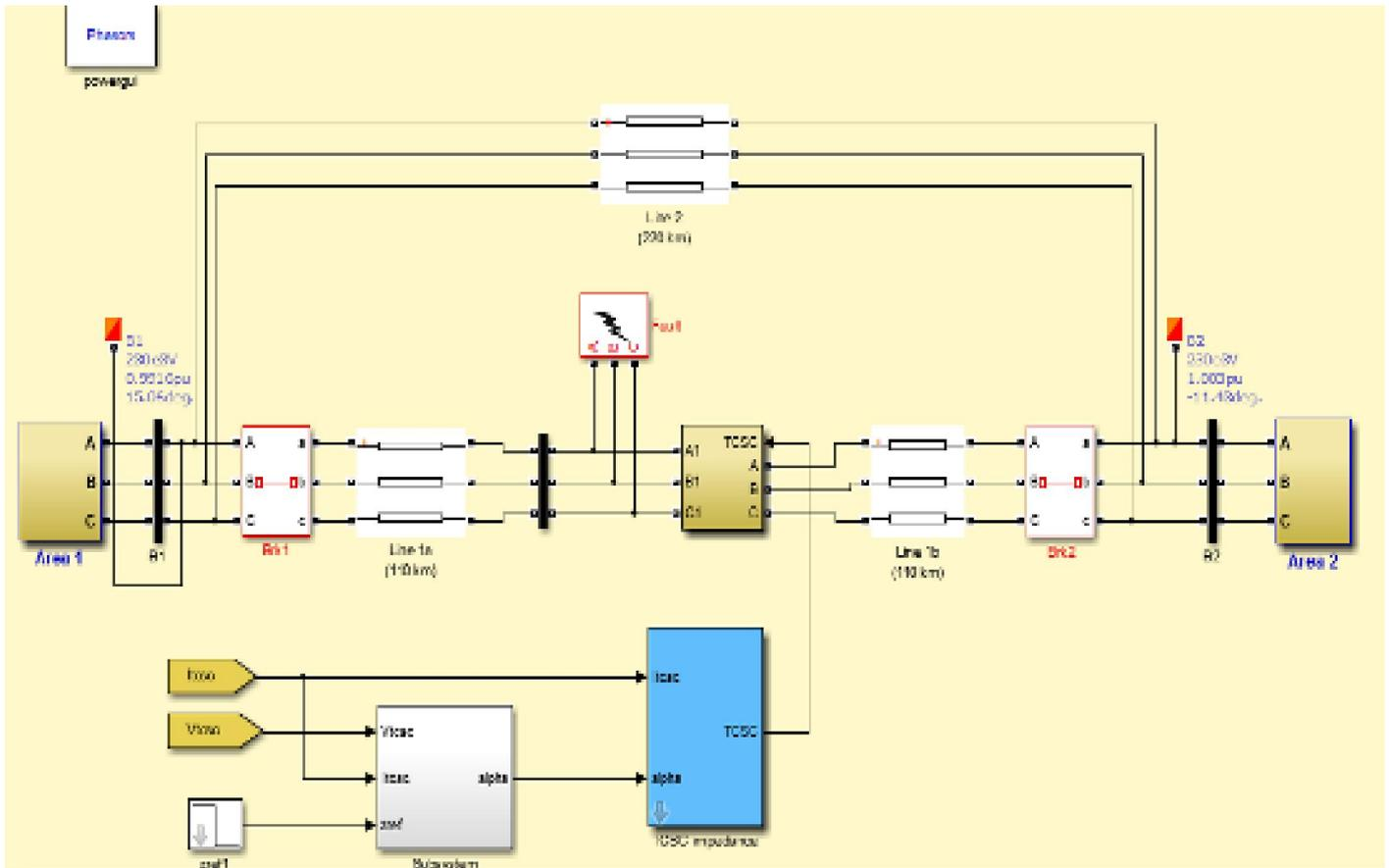
Fig. 7 Design of two area multi machine power system with TCSC.
