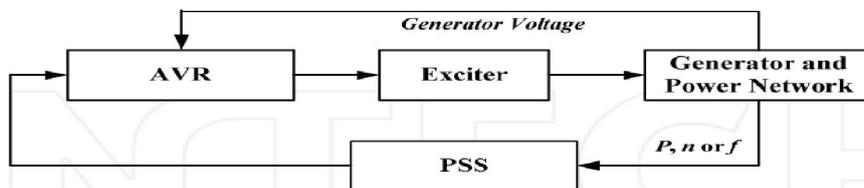
Fig.3 Structure diagram of power system stabilizer (PSS)
