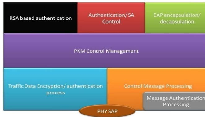
**Figure 2: WiMAX security sub layer**
