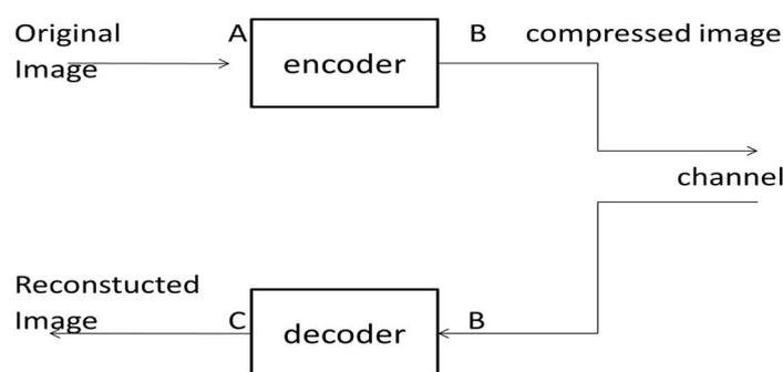
**Figure 1. Block diagram of image compression system**
